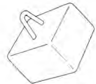
Cast or Concrete Sinker
