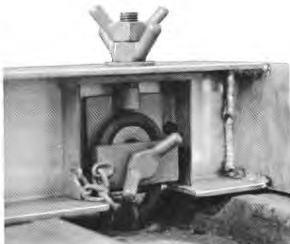
TIE-DOWN ASSY FOR ALUMINUM PORTABLE CAPSTAN
