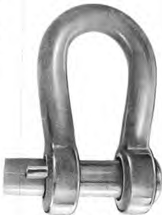
BOW SHACKLE WITH OVAL PIN AND FORELOCK KEY
