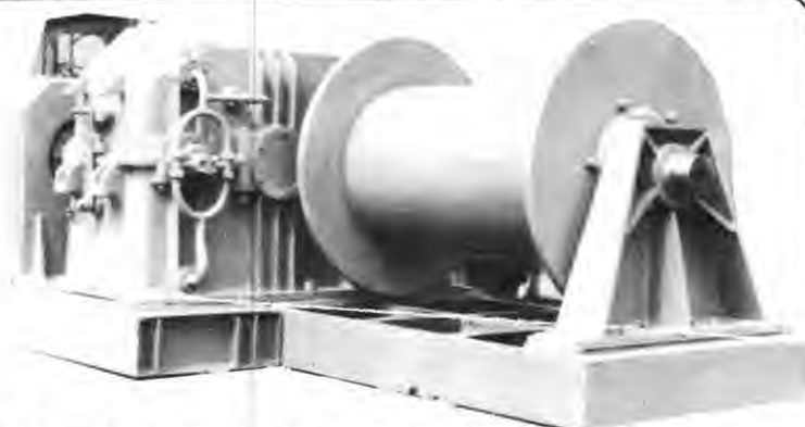
50/70 ton hydraulically driven Heavy-Lift Winch with drum to hold 1700m by 36mm diameter wire.
